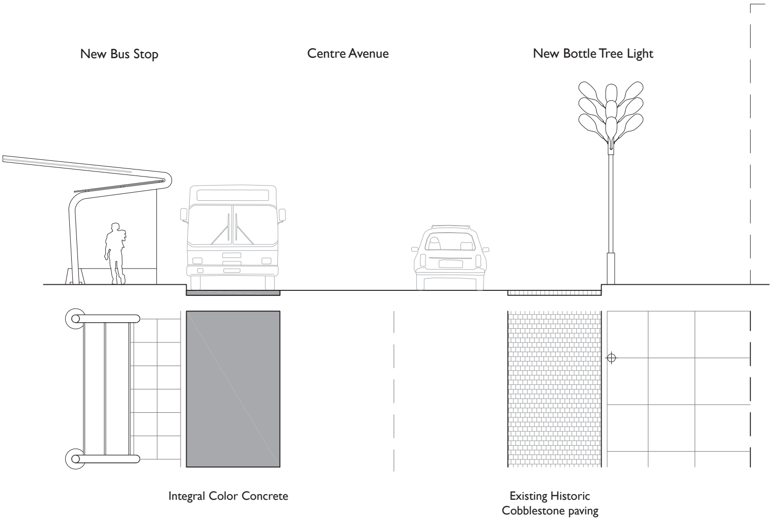
Typical Centre Avenue Section and Plan Detail A-A - Bus Shelter and Street Light Scale: 1/8" = 1'-0"
